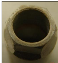
Nut w/ external corrosion
