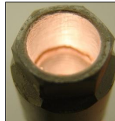
Nut w/ internal corrosion
