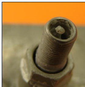
Unplated Valve Core, Corroded in Stem (Valve core will not actuate)
