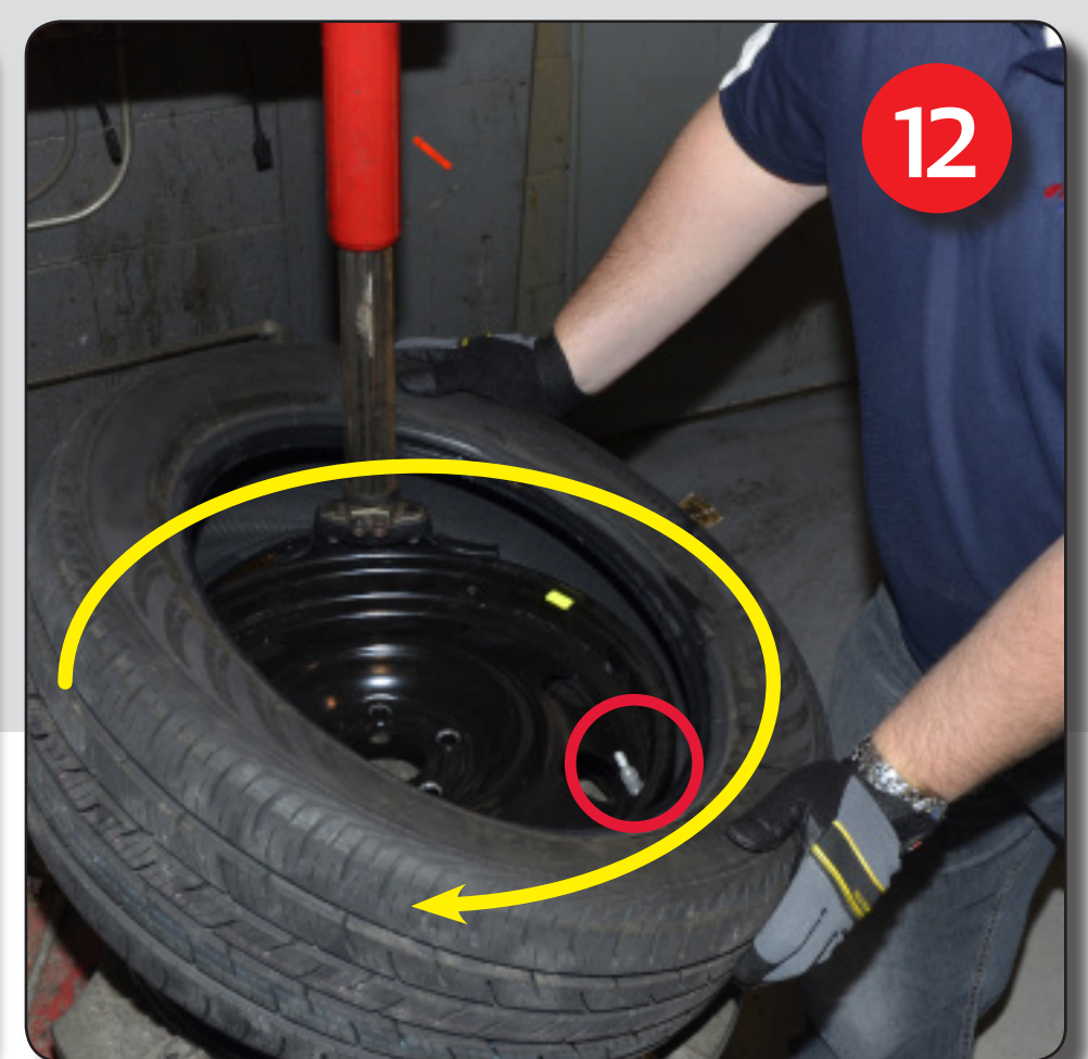
Tire installation - sensor installed (all sensor types)
