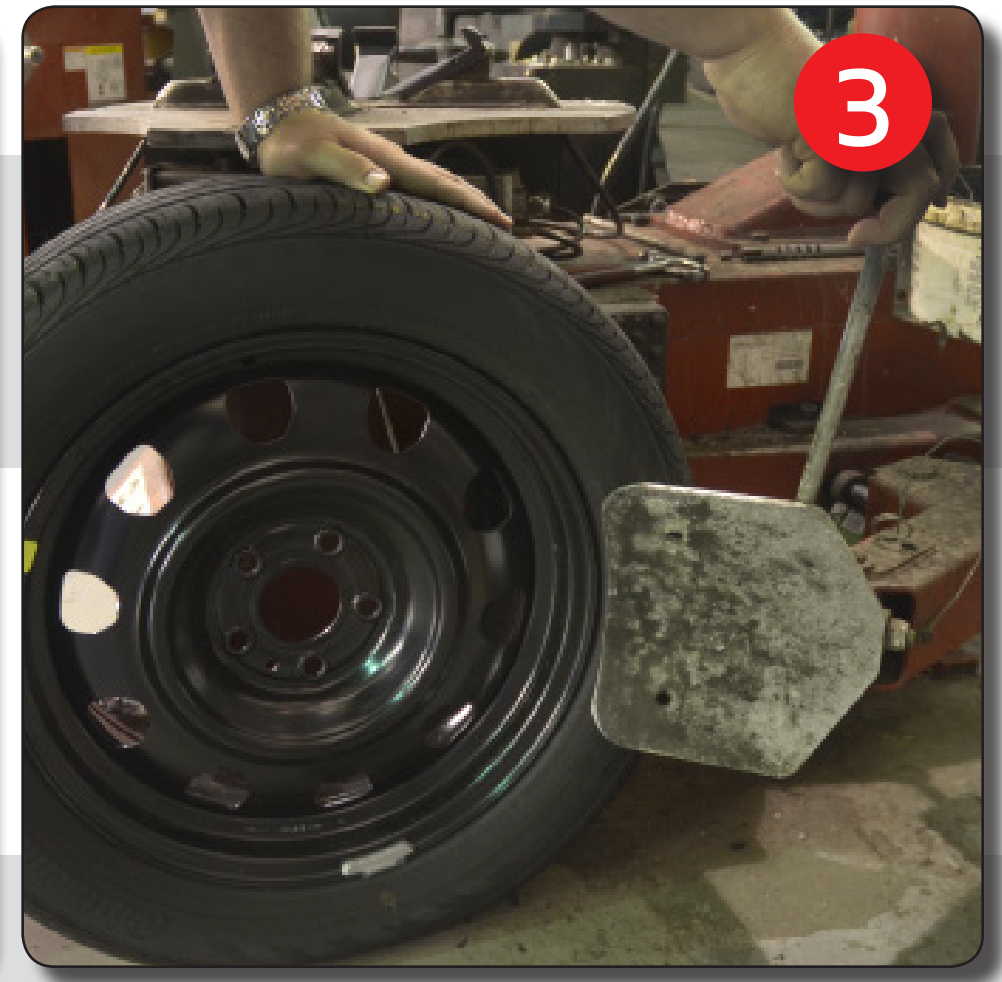
Breaking Bead with Sensor Removed
