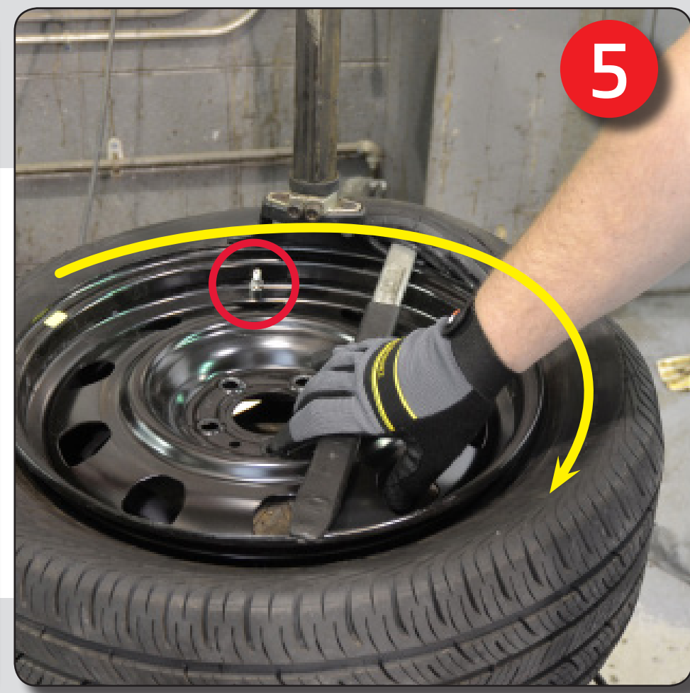
Mount/demount head just ahead of sensor
