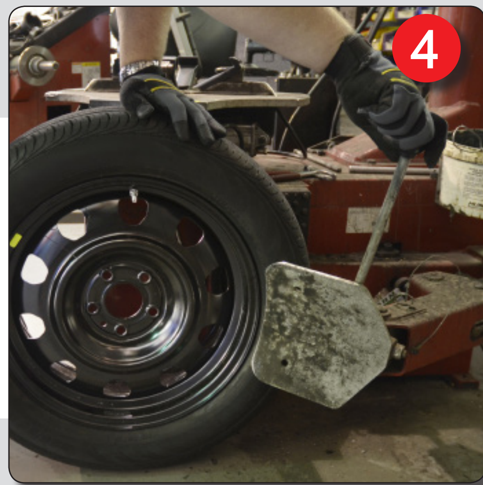
Break bead at 6 o'clock and 12 o'clock positions at all times
